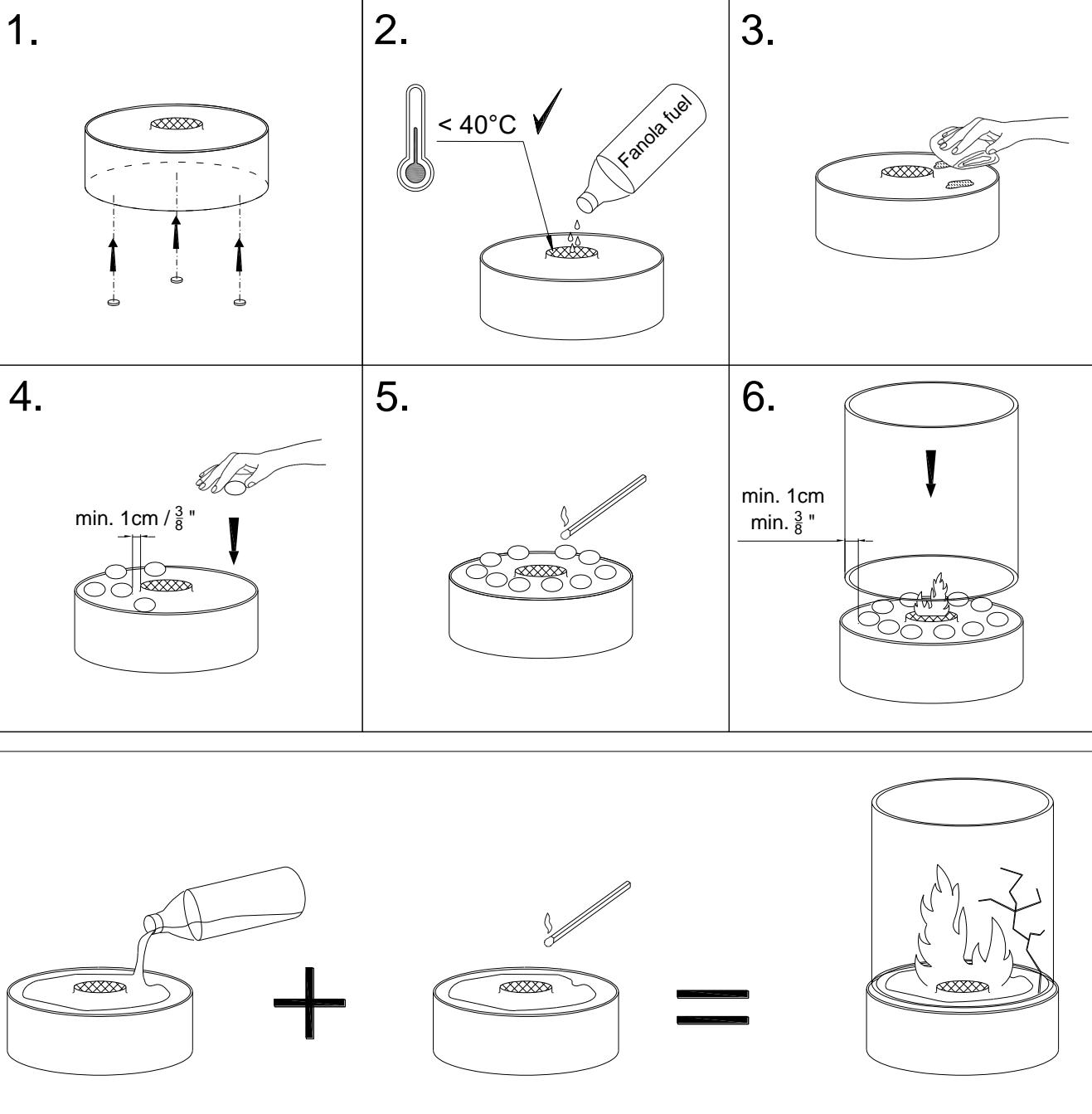
**EN** Igniting the spilled fuel is extremely dangerous and will cause the glass tube to crack. **Glass tube is not covered by the warranty.**
